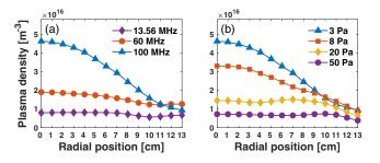
FIG. 2. Measured radial distributions of plasma density in an argon discharge (a) at different driving frequencies (3 Pa, 80 W) and (b) at different pressures (100 MHz, 80 W).
