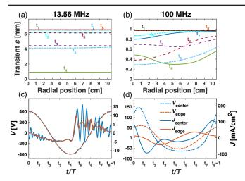
FIG. 3. Simulation results for discharges driven at 13.56 MHz (left) and 100 MHz (right) at 3 Pa, for a fixed power of 80 W. (a),(b) Sheath thickness s versus radius in eight equally spaced times over one rf cycle. (c),(d) Waveforms of the total discharge voltage V (dash-dotted lines) and total current density J (solid lines) at the electrode center (r=0) and edge (r=R), over one rf cycle.
