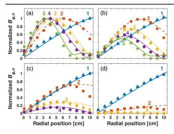
FIG. 4. Experimental data (points) and simulation predictions (lines) of the radial distributions of  $B_{\varphi,n}$  at different pressures: (a) 3 Pa, (b) 8 Pa, (c) 20 Pa, and (d) 50 Pa. All harmonic magnetic field amplitudes were normalized to the maxima at 3 Pa. Other conditions were  $\omega/2\pi=100$  MHz and power = 80 W.
