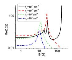
FIG. 4. (Color online). Surface resistance of warm bounded uniform Maxwellian plasmas for different electron densities as a function of the applied magnetic field. Discharge parameters: rf field frequency  $\omega/2\pi=29$  MHz, electron temperature  $T_e$ =4 eV, electron collision frequency  $\nu$ =1.2  $\times 10^7$  s<sup>-1</sup>, and the plasma half-length L/2=10.5 cm.
