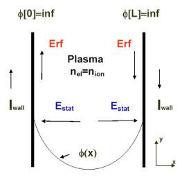
Fig. 1. 1-D model of bounded ICP. (Color version available online at http://ieeexplore.ieee.org.)
