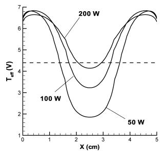
Fig. 9. Effective temperature profiles for a non-Maxwellian EEDF (solid lines) and a Maxwellian EEDF (dashed lines) for 1 mtorr [30], [40].
