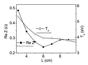
Fig. 4. Self-consistent simulations of the plasma surface resistance ReZ and the electron temperature  $T_e$  (defined as 2/3 of the average electron energy) at the discharge center as functions of the discharge gap. Discharge parameters are the coil current I = 5 A/cm, the RF field frequency  $\omega/2\pi = 13.56$  MHz and Argon pressure P = 3 mtorr [6].
