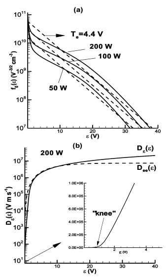
Fig. 8. (a) Self-consistently predicted non-Maxwellian (solid lines) and Maxwellian (dashed lines) electron energy distribution function (EEDF) as a function of total energy for 1 mtorr. (b) Energy diffusion coefficient [(2)]  $D_e(\varepsilon)$  (solid line) and energy diffusivity (see text) related to e-e collisions (dashed line) as a function of total energy for 1 mtorr. Inset shows an expanded scale for  $D_e(\varepsilon)$  [30], [40].
