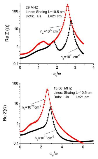
Fig. 25. Surface resistance as a function of a normalized electron–cyclotron frequency. Solid lines correspond to Shaing formalism for one grounded electrode with plasma length L. Dotted lines correspond to the case of two driving electrodes with plasma length 2L. Shown: RF driving frequency (a) 29 MHz (b) 13.56 MHz. Electron temperature  $T_e = 4$  eV, electron collision frequency  $\nu = 1.2 \ 10^7 \ s^{-1}$ . (Color version available online at http://ieeexplore.ieee.org.)
