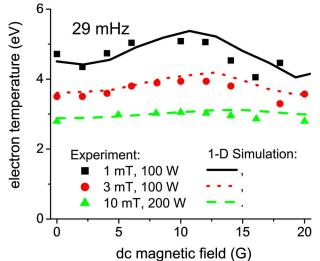
Fig. 22. Electron temperature at the discharge center as a function of the applied magnetic field for full self-consistent discharge simulations for different deposited powers and gas pressures. Case of one grounded electrode. Discharge parameters are the same as in Fig. 19. (Color version available online at http:// ieeexplore.ieee.org.)
