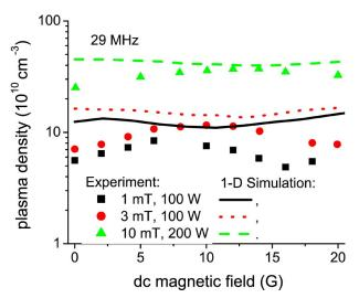
Fig. 23. Electron plasma density at the discharge center as a function of the applied magnetic field for full self-consistent discharge simulations for different deposited powers and gas pressures. Case of one grounded electrode. Discharge parameters are the same as in Fig. 19. (Color version available online at http://ieeexplore.ieee.org.)
