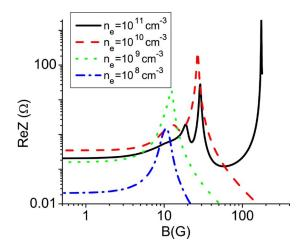
Fig. 16. Surface resistance of warm bounded uniform Maxwellian plasmas for different electron densities as a function of the applied magnetic field. Discharge parameters: RF field frequency  $\omega/2\pi = 29$  MHz, electron temperature  $T_e = 4$  eV, electron collision frequency  $\nu = 1.2 \ 10^7 \ s^{-1}$ , and the plasma half-length L/2 = 10.5 cm [33]. (Color version available online at http://ieeexplore.ieee. org.)
