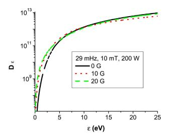
Fig. 20. Energy diffusion coefficient as a function of the electron energy for full self-consistent discharge simulations for different applied magnetic fields. Case of one grounded electrode. Discharge parameters are the same as in the Fig. 19. (Color version available online at http://ieeexplore.ieee.org.)
